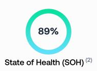
Remaining usable capacity / Usable capacity when new (3)
